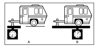
If you're using a weigh-carrying hitch or a weight-distributing hitch, the trailer tongue (A) should weigh 10 to 15 percent of the total loaded trailer weight (B).
